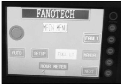
**Touch Screen Control.** Allows the operator to monitor the operation of the compactor and to change operating parameters of the machine on the screen.
