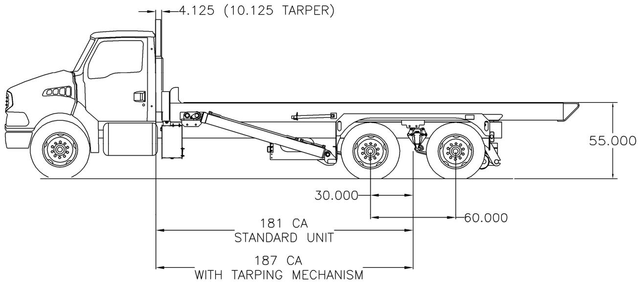
Typical Layout 23' 6" Hoist with or without Tarper System
